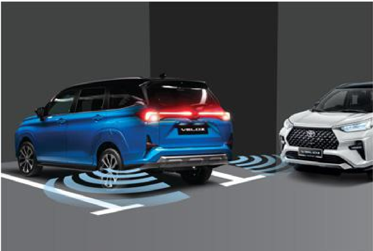
Rear Cross Traffic Alert (RCTA) Assists the driver when in reverse.
